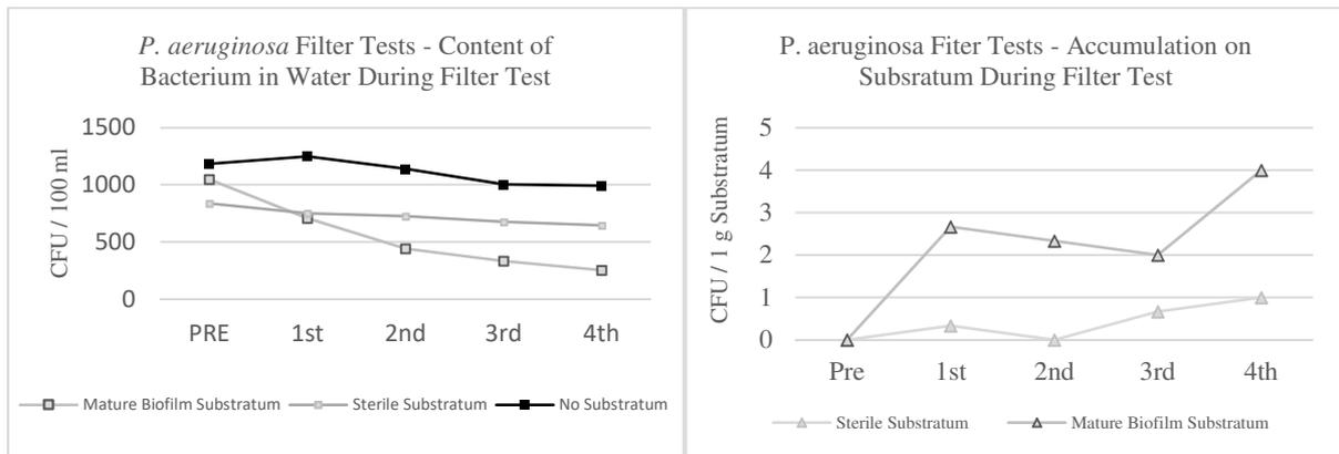
**Figure 2.** Inoculated water was filtered 4 times (n=9). Samples from the water were taken after each filter pass. Mature biofilm substratum consistently showed significant amounts of *P. aeruginosa* removed from the water. The mature substratum reduced *P. aeruginosa* water content by 76 % after 4 passes). While, the sterile substratum showed a reduction of 24 % after four passes (reduction of 192 CFU after 4 passes).
