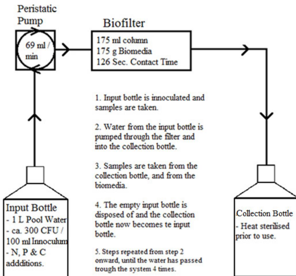
**Figure 1.** The experiment was set up as shown. The image in this figure details phase 1 of the experiment. This phase was followed by phase 2, where the contaminated water was replaced with uncontaminated water, which was circulated, before being sampled and replaced again - showing rate sheering from the substrate each subsequent 24 hours post-contamination.
